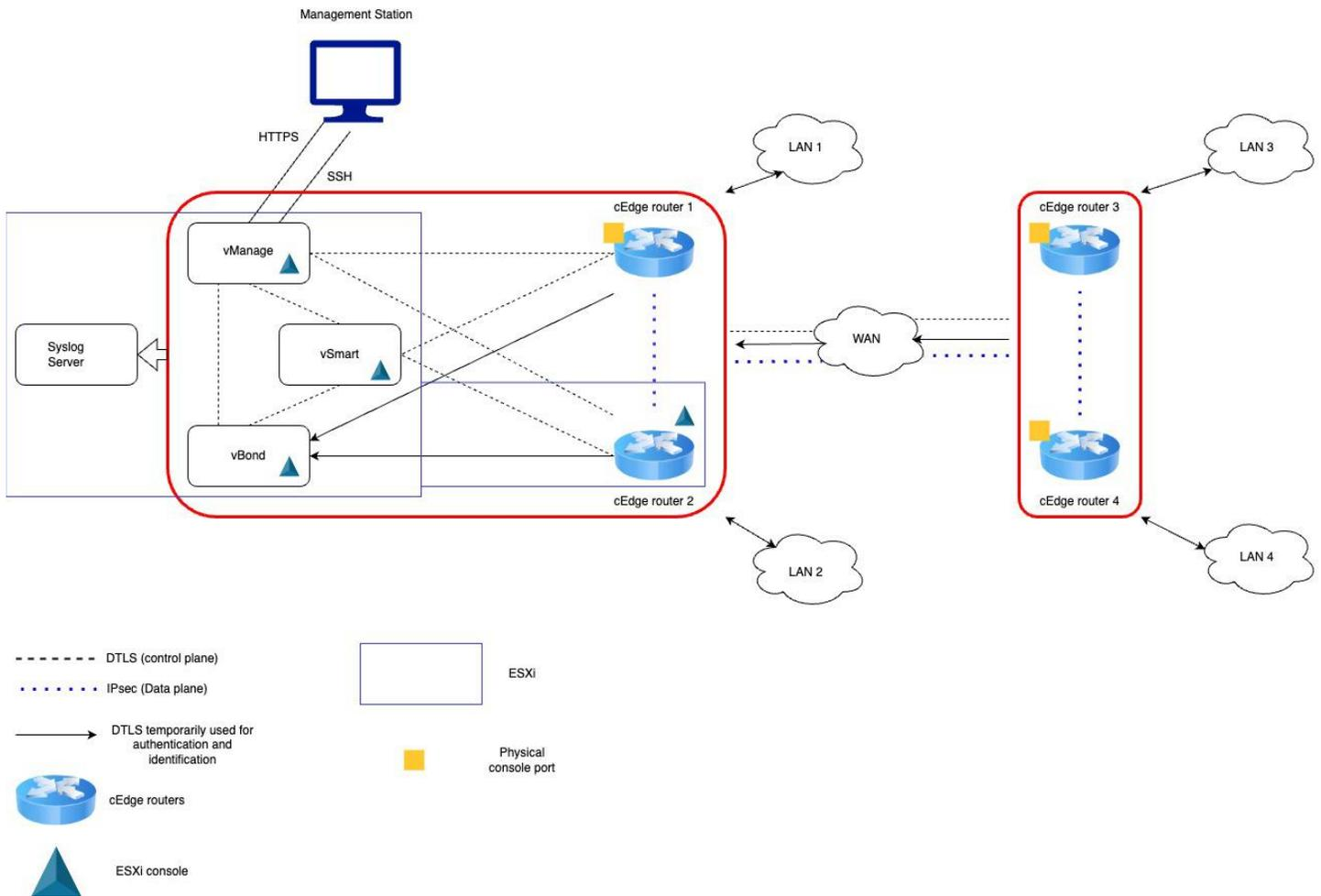
Figure 1: TOE Architecture
